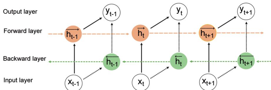
Fig. 3. Structure of the neural network BIGRU.
