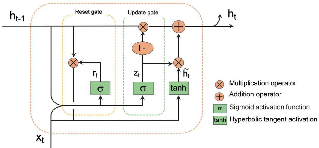
Fig. 2. Structure of GRU unit.
