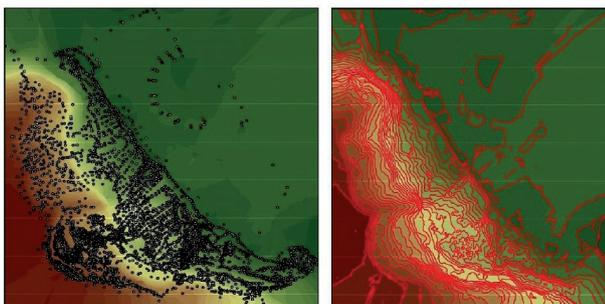
Fig. 3. Highlight of GPS measurement points (left); lines, generated of the point data (right).
