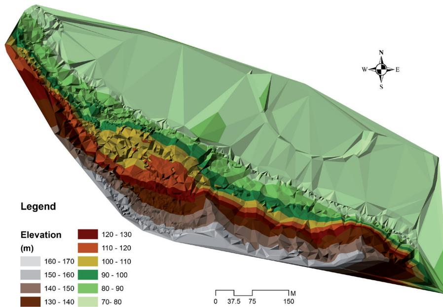
Fig. 11. Breasta landslide – altimetric model (TIN).
