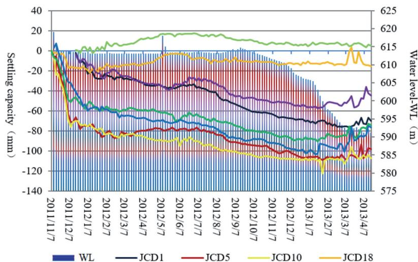
Fig. 7. The relationship curve between subsidence displacement with frontal reservoir water level.
