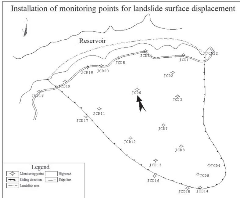
Fig. 3. Location layout of monitoring points.
