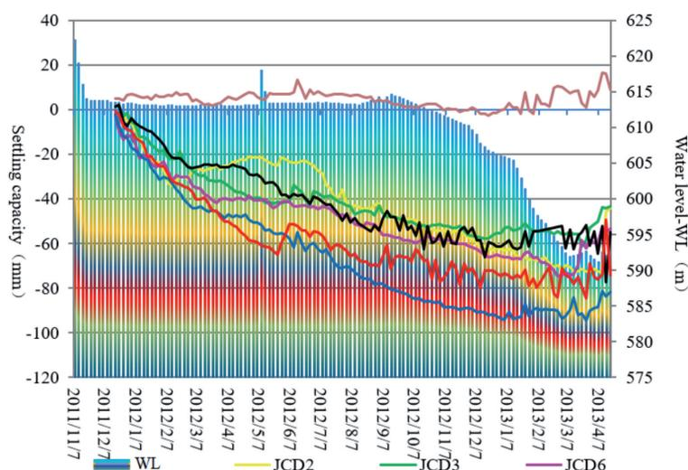
Fig. 8. The relationship curve between subsidence displacement with rainfall and middle reservoir water level.
