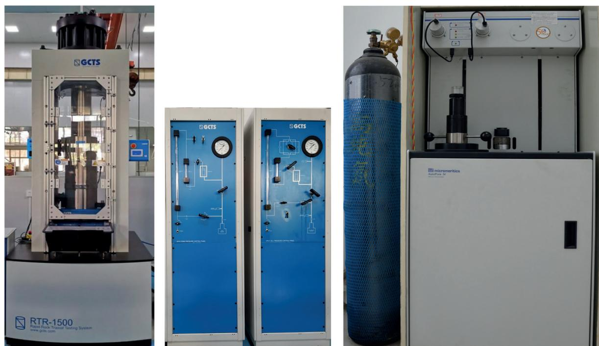
Fig. 5. Experimental equipment diagram: a RTR-1500 rapid triaxial rock testing system, b Mercury porosimeter.
