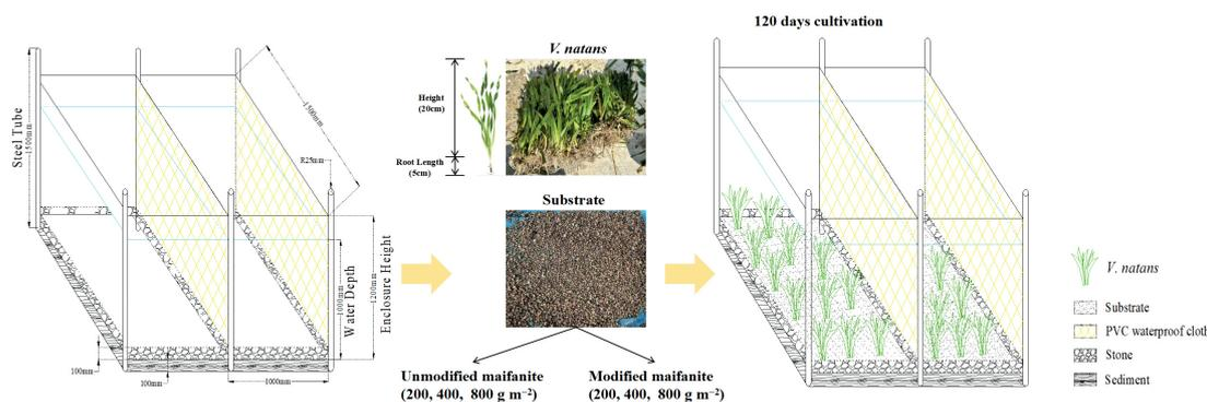
Fig. 1. Experimental set-up.
