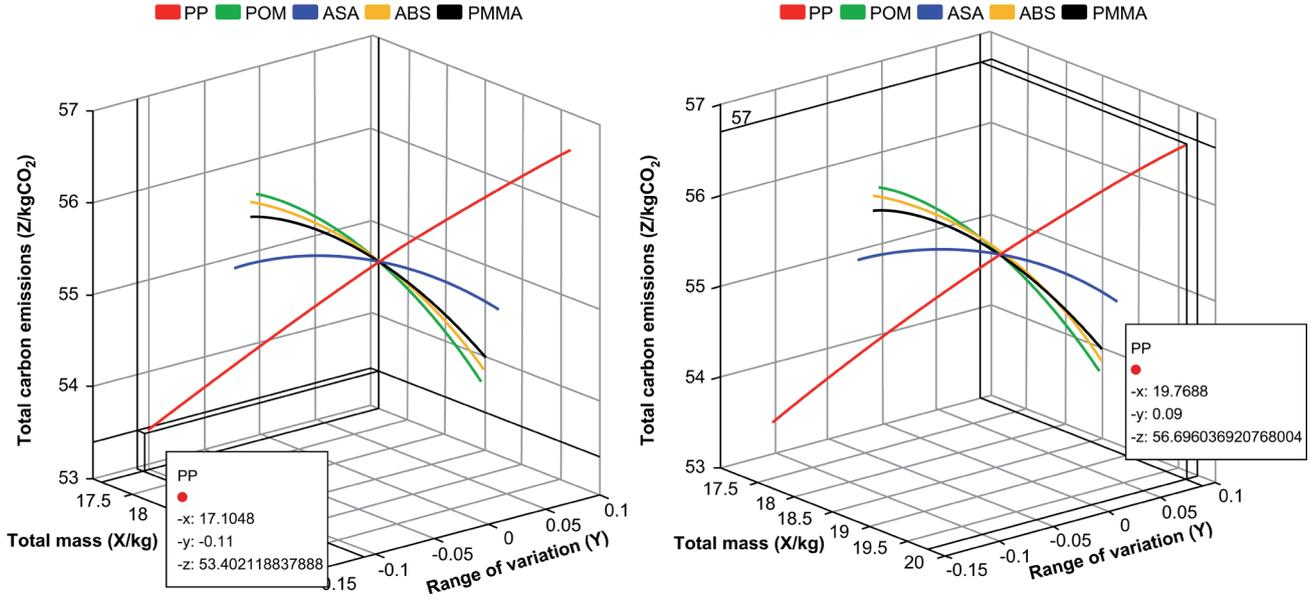
Fig. 4. Range of changes in total carbon emissions with changes in the mass share of five materials.
