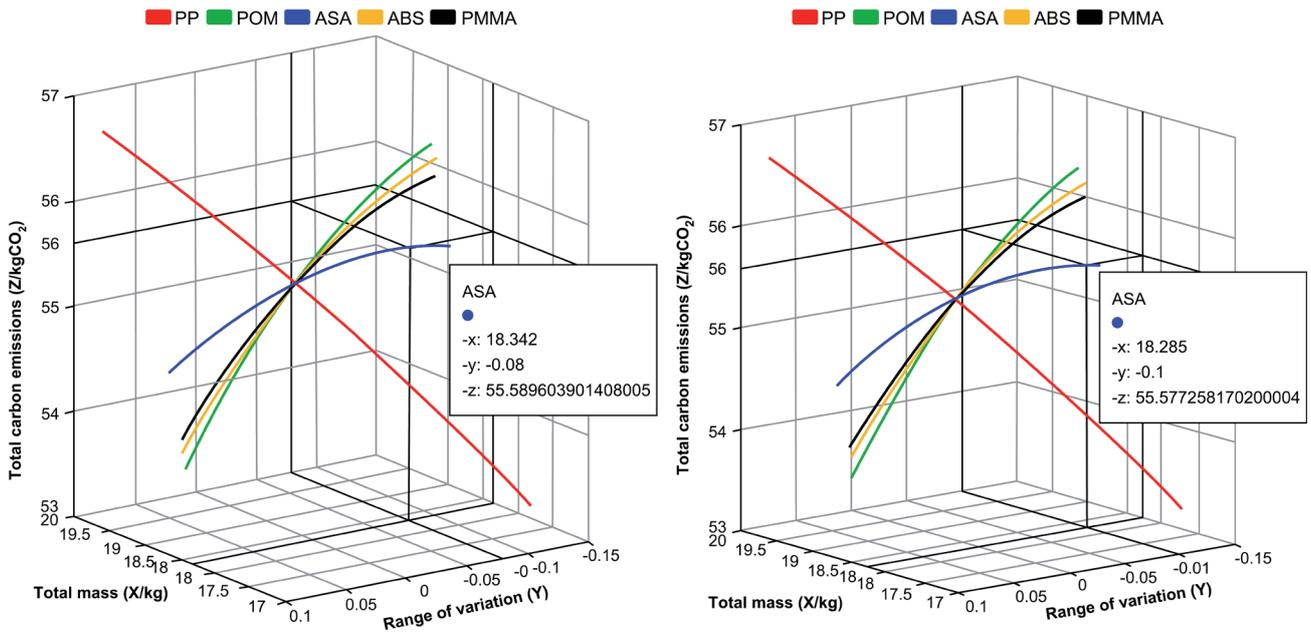
Fig. 5. Carbon emission extremes for ASA material changes.
