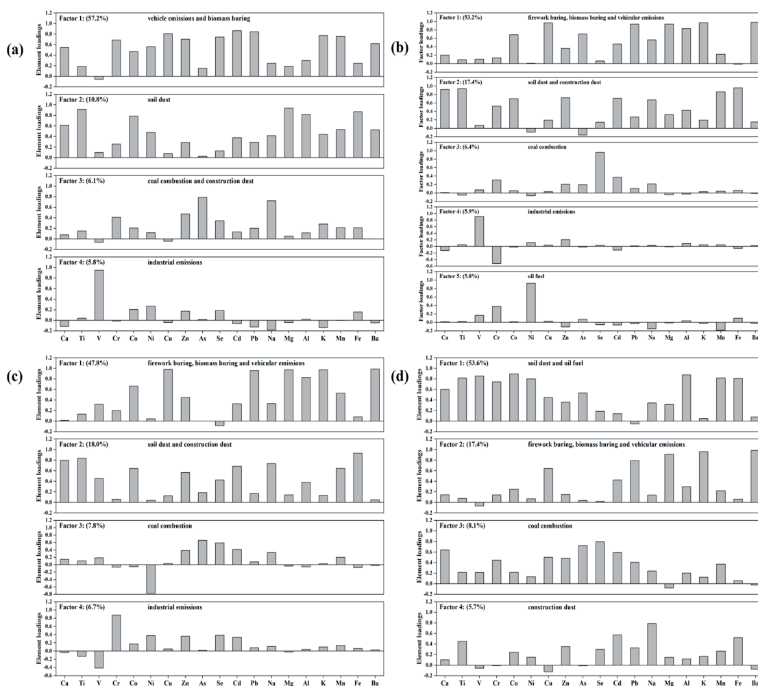
Fig. 8. Varimax-rotated principal component loading for elements in PM_{2.5} in SQ a), in GP b), in JL c), and GH d).
