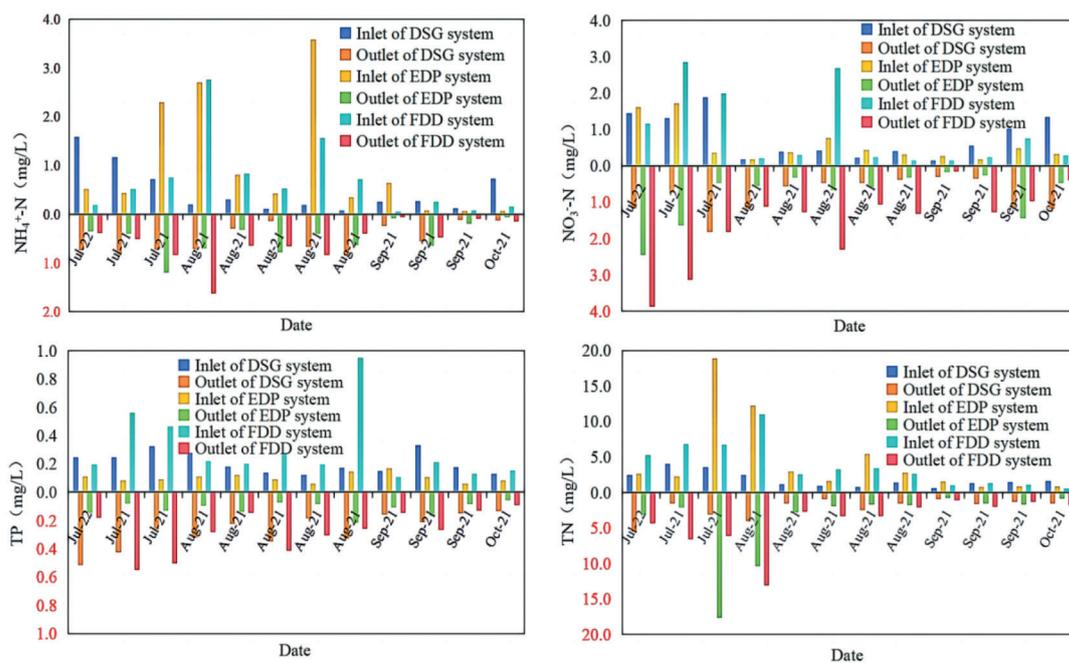
Fig. 5. Changes in N and P pollutants concentrations at the inlet and outlet in different drainage systems.
