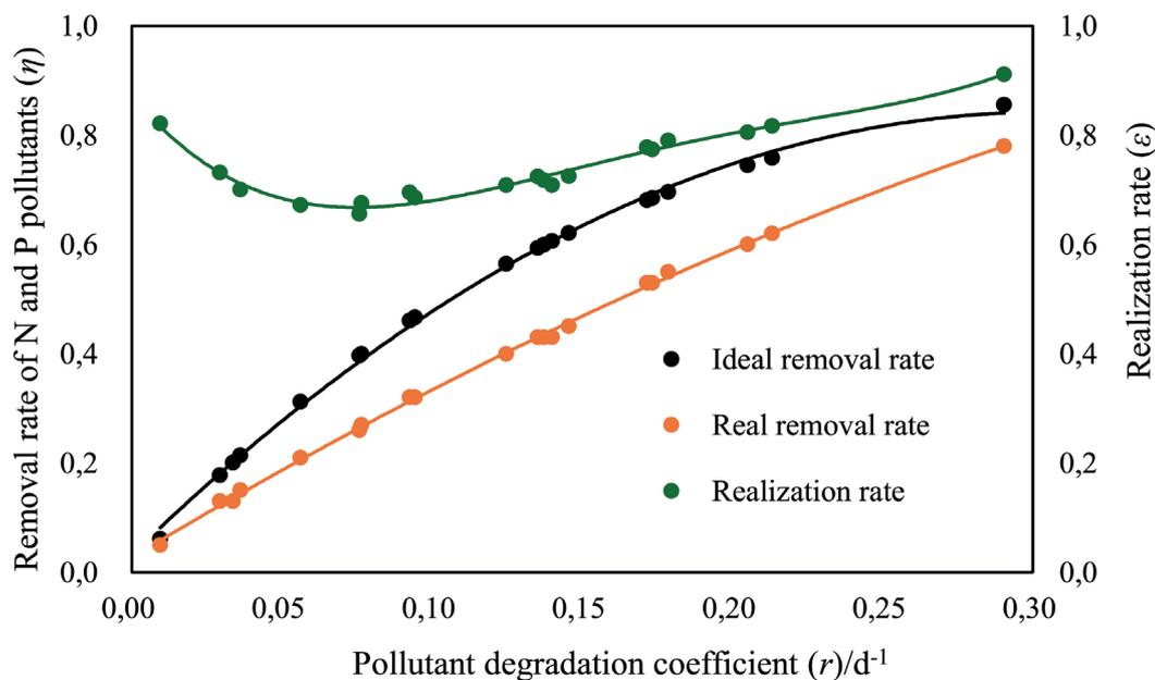
Fig. 6. Variations of pollutant removal rate with degradation coefficient in ditches and ponds under different hydraulic conditions.
