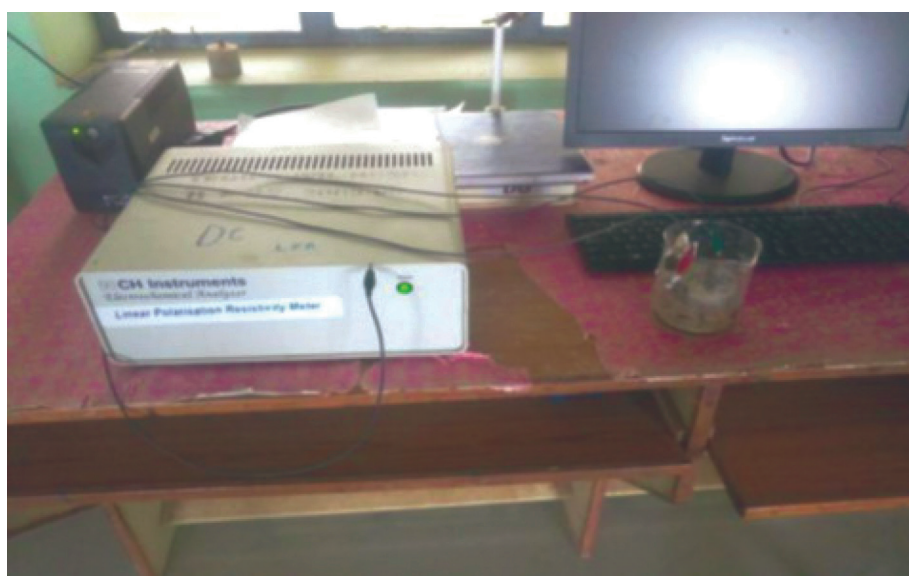
Fig. 6. Test set up for corrosion rate.
