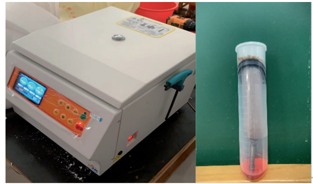
Fig. 3. Diagram of centrifuge and homemade centrifuge tube setup.
