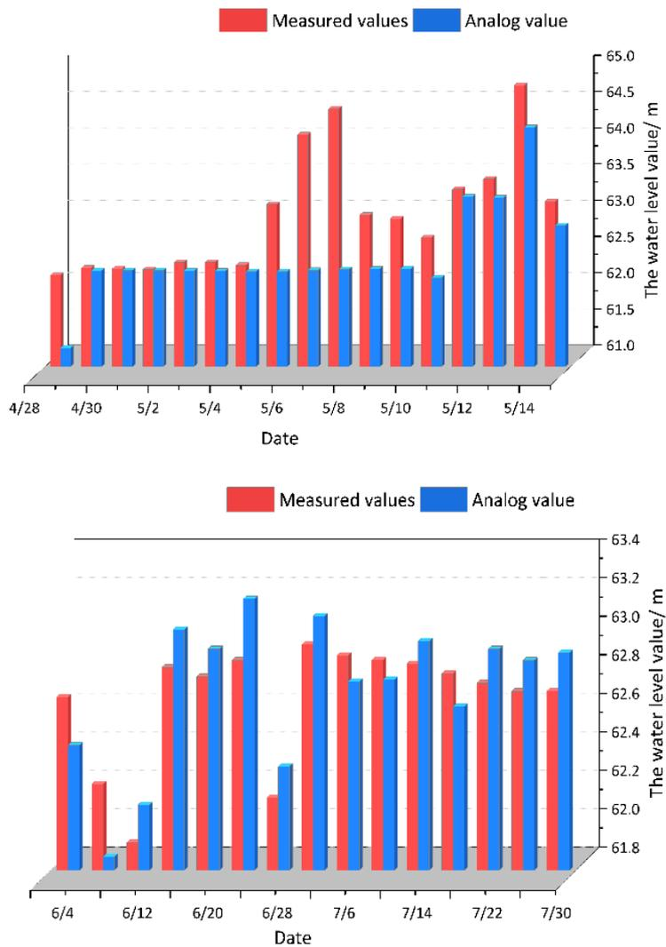
Fig. 11. Verification results of Lugou Bridge in 2020 and 2021.
