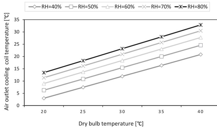
Fig. 7. Variation of design air outlet from evaporator with dry bulb temperature for different relative humidities.
