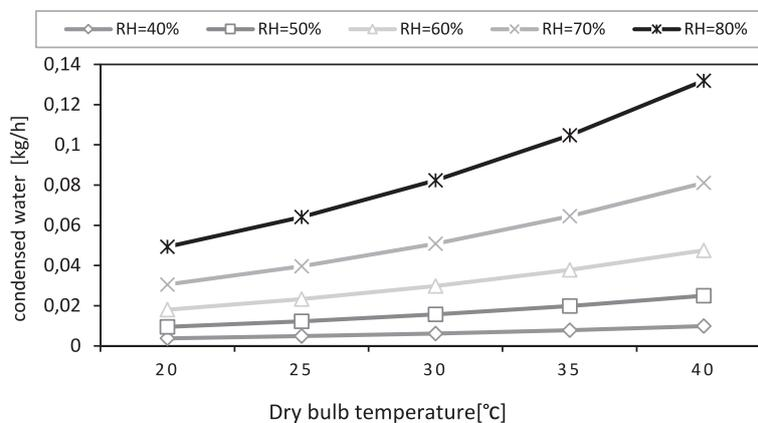
Fig. 6. Variation of water condensation rate with dry bulb temperature for different relative humidities for 5 kW evaporator cooling capacity.
