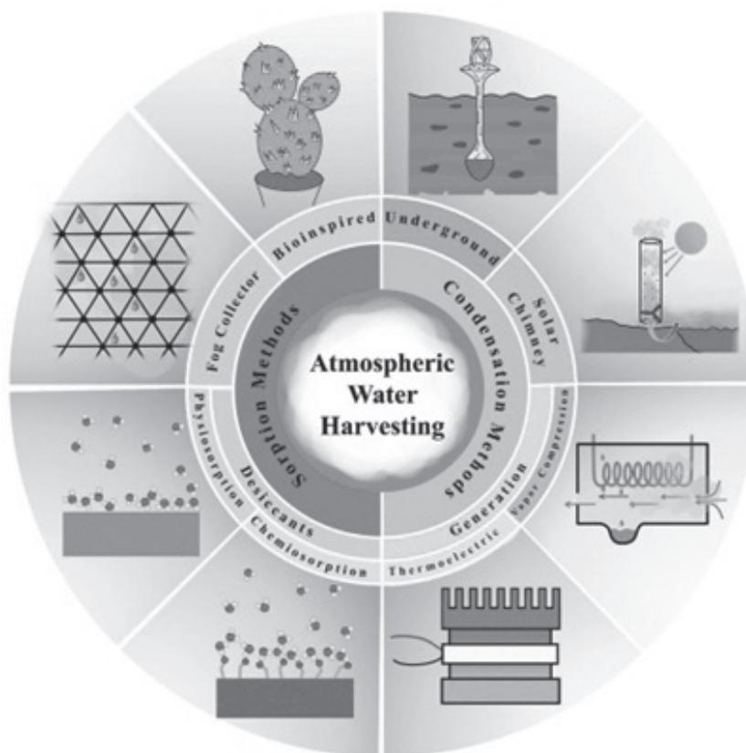
Fig. 1. Techniques for atmospheric water extraction [32].
