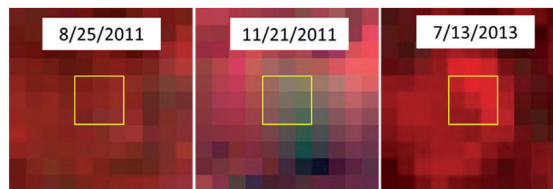
Fig. 10. Omission error of detecting disturbance agent (clearcut) within a 3 \times 3 spatial window (yellow boxes) using the AEWMA-t algorithm: the extremely sparse clear observations during disturbance. The dates corresponding to three dashed lines in AEWMA-t chart correspond to those of Landsat images in turn.
