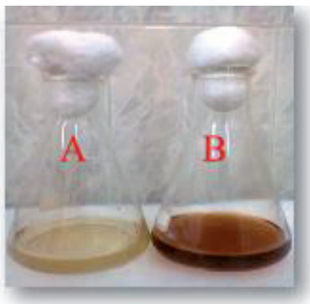
Fig. 3. Preparation of AgNPs using P. expansum (A) Cell-free extract of P. expansum (B) Color change after incubation of P. expansum cell-free extract with silver nitrate.
