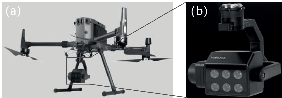
Fig. 3. Image acquisition platform: (a) DJI M300RTK Unmanned Aerial Vehicle; (b) MS600 Pro multispectral camera.
