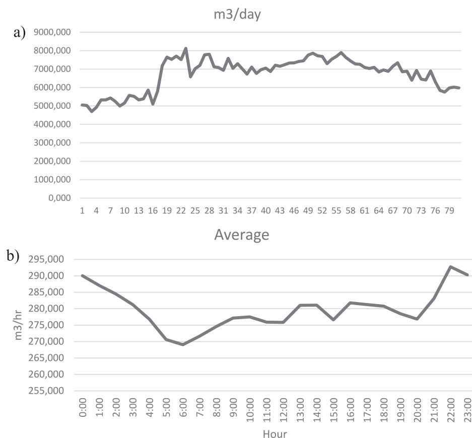
Fig. 4. a) Volume of wastewater generated over the 81-day study period, b) hourly flow rates for the study duration.
