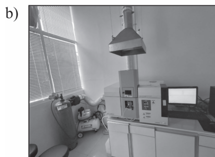
Fig. 6. Measurement of lead concentration in water: a) solution filtration, b) analysis using AAS.
