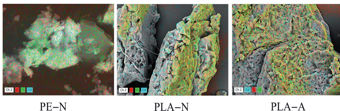
Fig. 6. Cd elemental mapping on the surface of MPs after adsorption (SEM-EDS).
