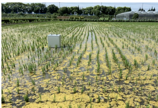
Fig. 3. Static chamber N 2 O sampling and rice cultivation experiment.
