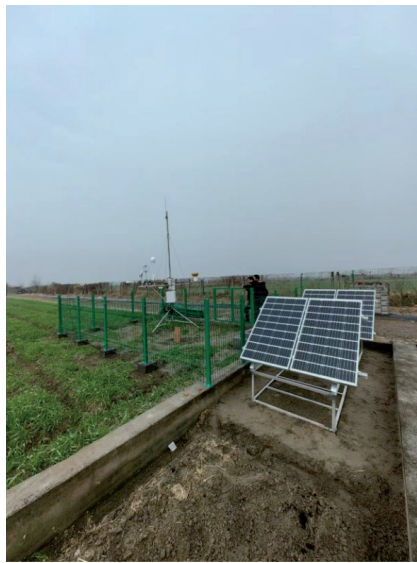
Fig. 2. Open-path greenhouse gas flux monitoring system.
