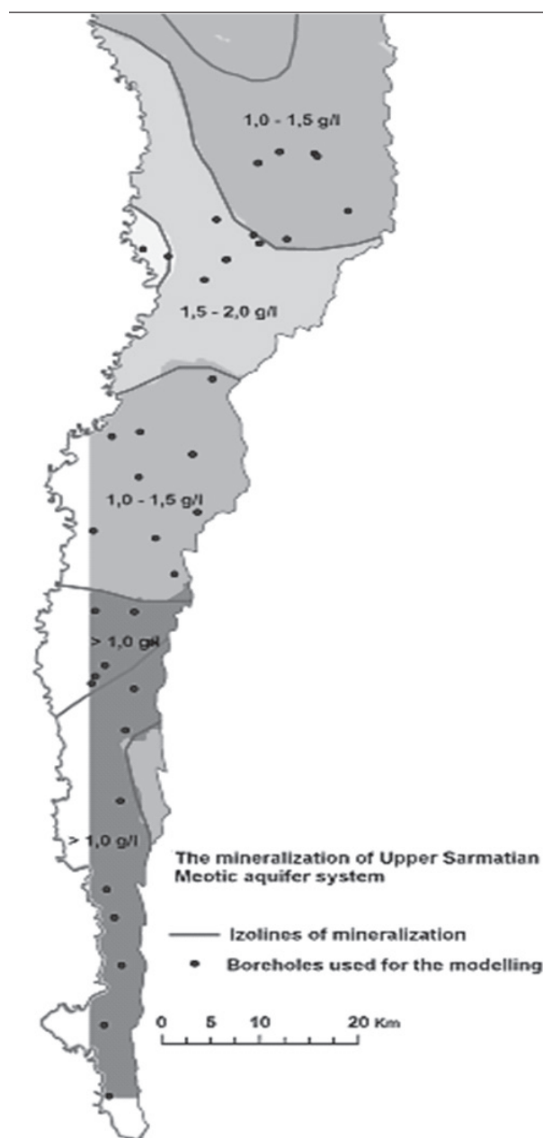
Fig. 4. Mineralization of the Upper-Sarmatian aquifer in the southern part of the Prut River Basin [13].
