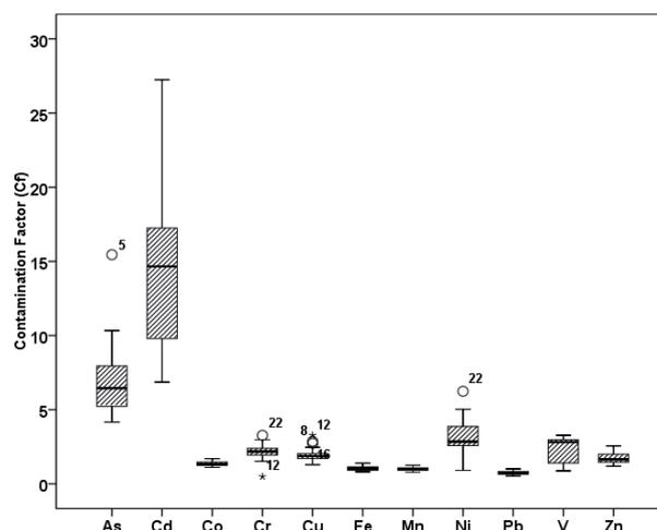
Fig. 4. Contamination factor (Cf) of heavy metals plotted in box and whisker method (rectangle-contamination factor of metals; central line of each plot-median) of the surface sediments of Namal Lake.
