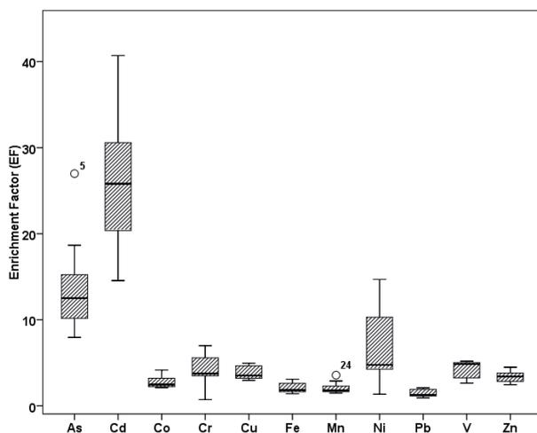
Fig. 2. Enrichment factor (EF) of heavy metals plotted in box and whisker method (rectangle-enrichment of metals; central line of each plot-median) of the surface sediments of Namal Lake.
