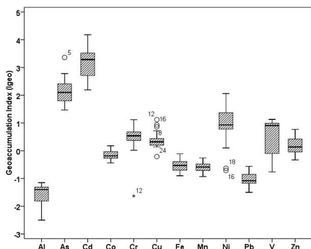
Fig. 3. Geo-accumulation index (Igeo) of heavy metals plotted in box and whisker method (rectangle-geo-accumulation index of metals; central line of each plot-median) of the surface sediments of Namal Lake.
