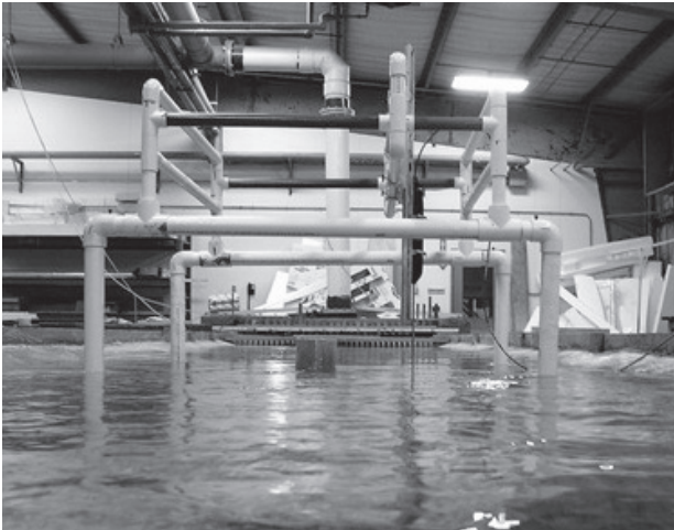
Fig. 1. ADV mounted on a plastic frame that is movable for three axes.
