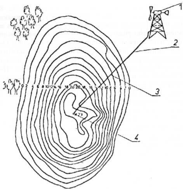
Fig. 2. Starodworskie Lake: 1 - wind turbine, 2 - steel air pipeline, 3 - flexible air pipeline, 4 - aerator.
