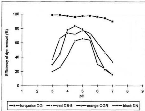
Fig. 5. Effect of pH on efficiency of dye removal.
