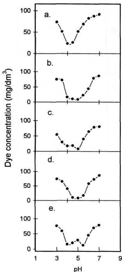
Fig. 4. Effect of pH and coagulant dosage on concentration of black DN after coagulation; a - 0.3 mg Al/mg dye, b - 0.5 mg Al/mg dye, c - 0.8 mg Al/mg dye, d - 1 mg Al/mg dye, e - 2 mg Al/mg dye.
