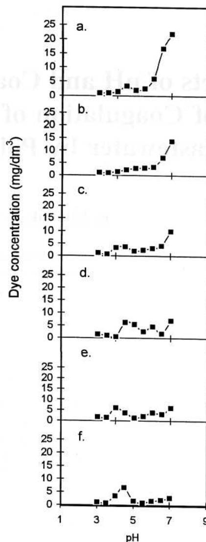
Fig. 1. Effect of pH and coagulant dosage on concentration of turquoise DG after coagulation; a - 0.3 mg Al/mg dye, b - 0.5 mg Al/mg dye, c - 0.8 mg Al/mg dye, d - 1 mg Al/mg dye, e - 2 mg Al/mg dye, f - 3 mg Al/mg dye.
