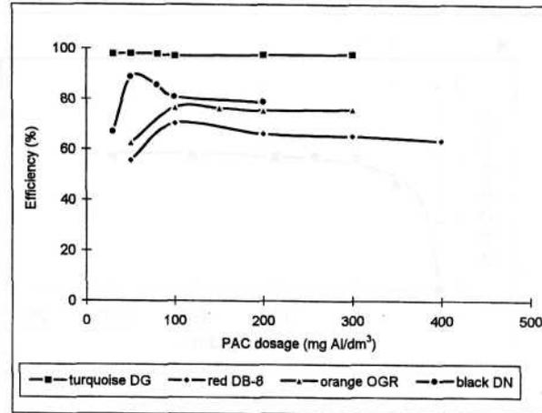
Fig. 6. Effect of coagulant dosage on efficiency of dye removal.
