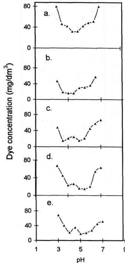
Fig. 3. Effect of pH and coagulant dosage on concentration of orange OGR after coagulation; a - 0.5 mg Al/mg dye, b - 1 mg Al/mg dye, c - 1.5 mg Al/mg dye, d - 2 mg Al/mg dye, e - 3 mg Al/mg dye.
