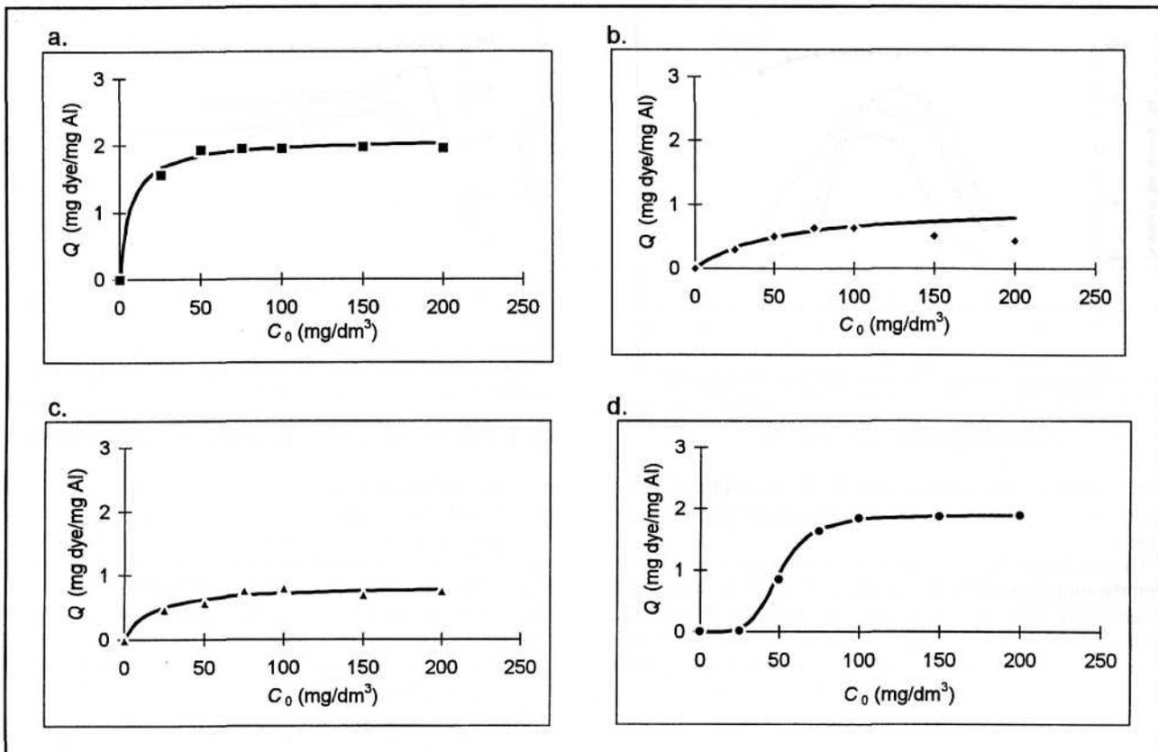
Fig. 7. Effect of initial dye concentrations ( $C_0$ ) on dye removal ( $Q$ ); a, b, c - Langmuir isotherms for turquoise DG, red DB-8, orange OGR, d - modified Langmuir isotherms for black DN.
