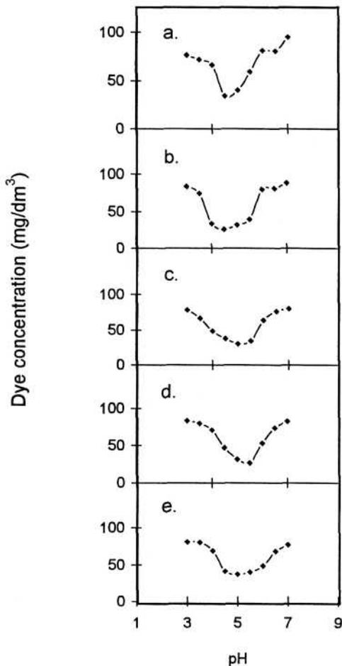
Fig. 2. Effect of pH and coagulant dosage on concentration of red DB-8 after coagulation; a - 0.5 mg Al/ mg dye, b - 1 mg Al/mg dye, c - 2 mg Al/mg dye, d - 3 mg Al/mg dye, e - 4 mg Al/mg dye.
