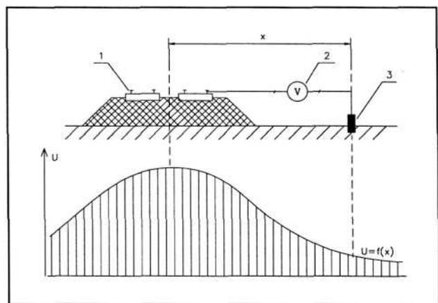
Fig. 3. Potential measurement of electric traction rails: 1 - rail, 2 - voltmeter, 3 - reference electrode.
