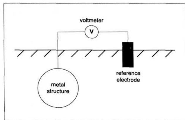
Fig. 1. Potential measurement of structures.
