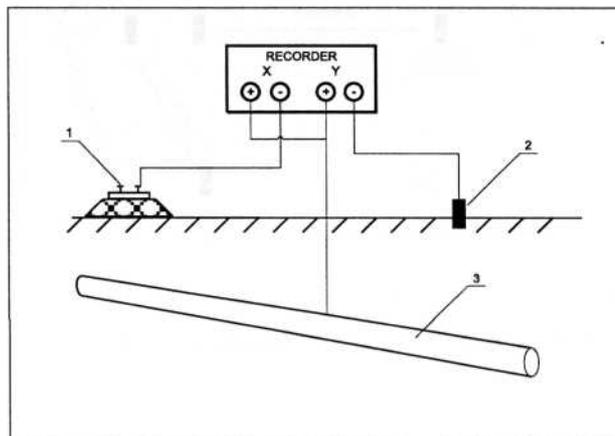
Fig. 4. Method of connection of a recorder to the rail (1), reference electrode (2) and pipeline (3) for measurements by the correlation method.
