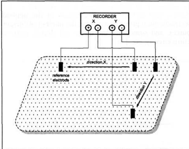
Fig. 2. Measurement of electric field distribution in the ground.
