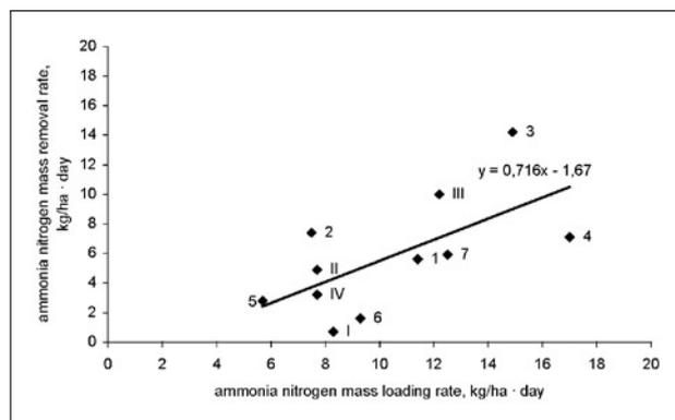
Fig. 2a. Ammonia nitrogen mass loading and removal rates in HF-CW household system.
