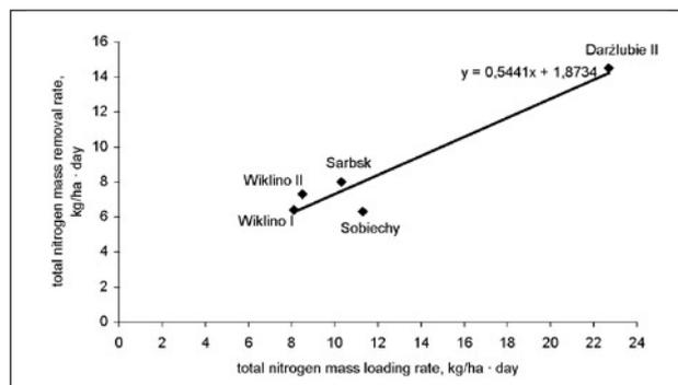
Fig. 6. Total nitrogen mass loading and removal rates in studied hybrid systems.
