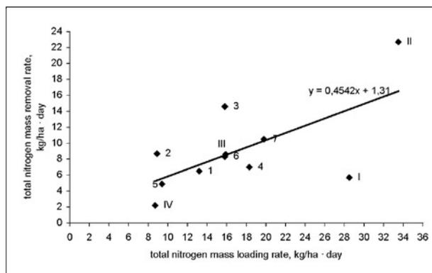
Fig. 2b. Total nitrogen mass loading and removal rates in HF-CW household system.
