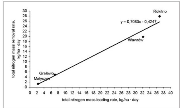
Fig. 4b. Total nitrogen mass loading and removal rates in local HF-CWs near Gorzów, Poland.
