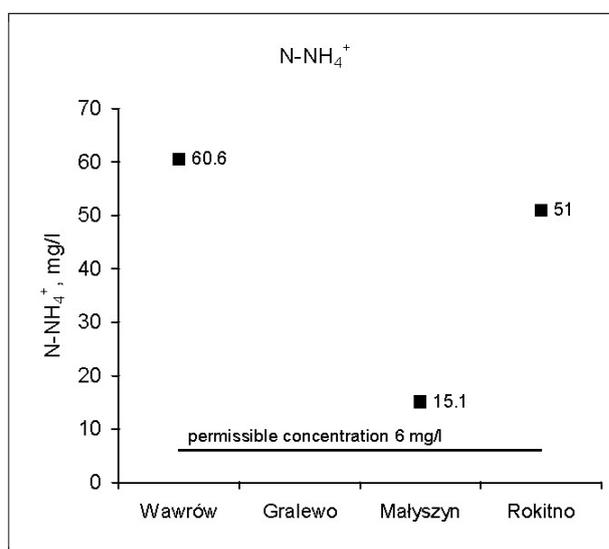
Fig. 3. Average concentration of ammonia nitrogen and total nitrogen in the effluent in local HF-CWs near Gorzów, Poland.
