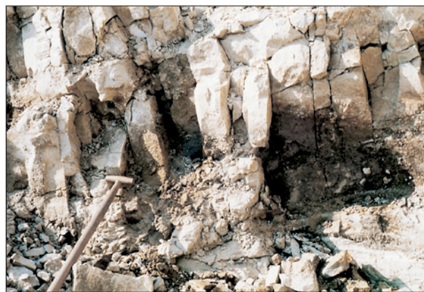
Fig.2. The bedrock opoka at approximately 5 m depth, appearing at this place in vertical layers.
