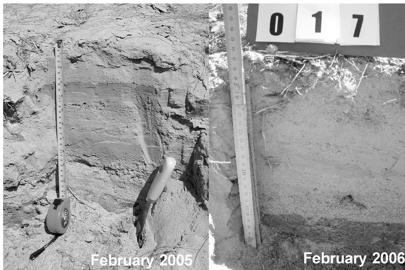
Fig.15. Over 20 cm thick layer of tsunami sediments composed of three upward fining sequences observed shortly after the tsunami (February 2005) and over one year later (February 2006). The sedimentary record is well preserved. Locations: Ban Bang Sak I.
