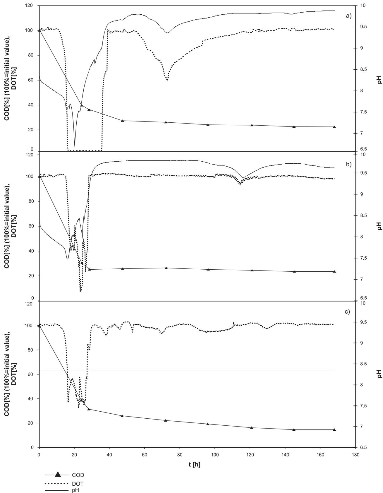
Fig. 5. Variations in the parameters chosen during the biodegradation of vinasse in the STR.
