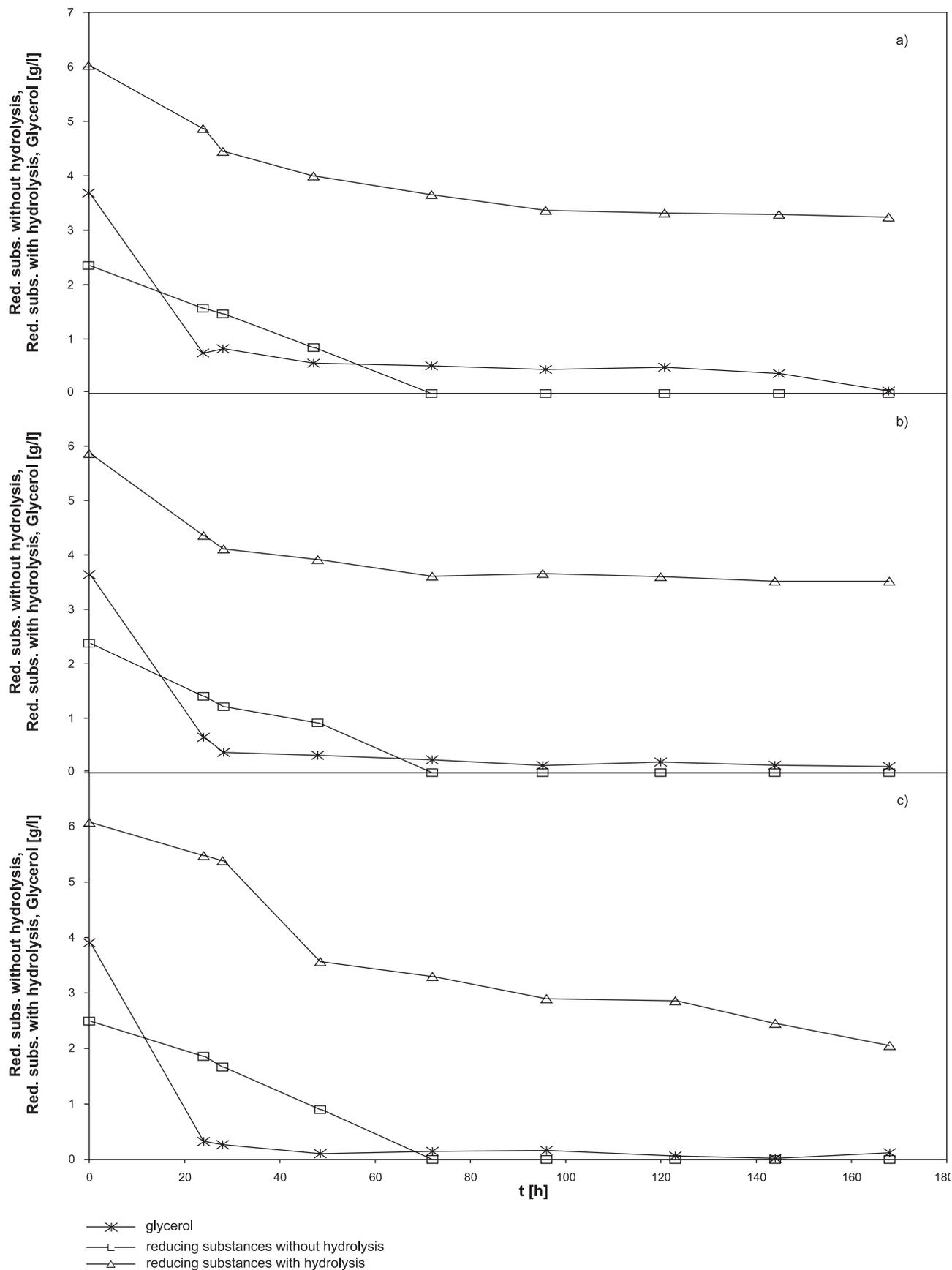
Fig. 7. Variations in the concentration of glycerol and the reducing substances during biodegradation of vinasse in the STR.
