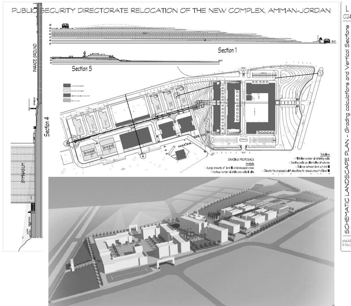
Fig. 4. During the landscaping of the PSD complex, existing topographic conditions were assessed to modify the architectural project; the aim was to lower the application costs. The architectural plan proposes large volumes of cut and fill; we illustrated a new plan for the development with minor changes of spot elevations. The solutions to grading problems were displayed as several vertical sections.
