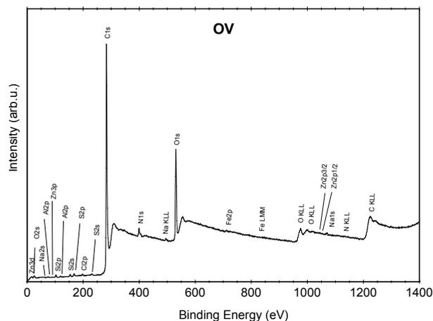
Fig. 4. Example of the XPS spectrum for the PM10 sample from “CROSSROADS” (May10-11).
