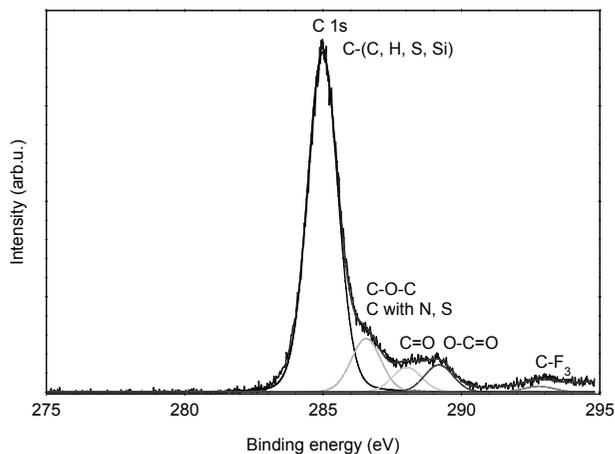
Fig. 8a. Carbon spectral line in narrow energy bandwidth 275 – 295 eV for PM2.5 sampled on August 10-11, 2005, at “BACK-GROUND.”
