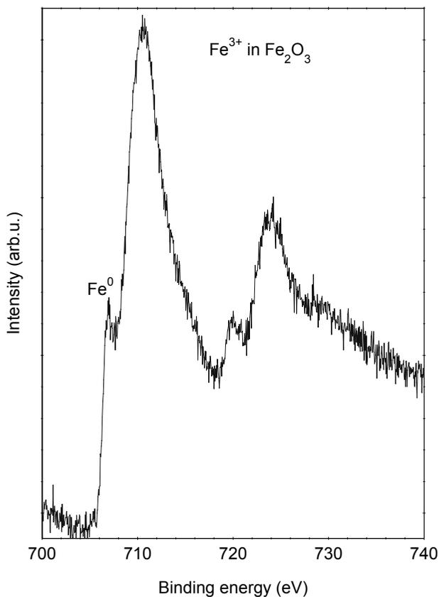
Fig. 10. Iron spectral line in narrow energy bandwidth 700 – 740 eV for PM2.5 sampled on August 10-11, 2005, at “CROSSROADS.”
