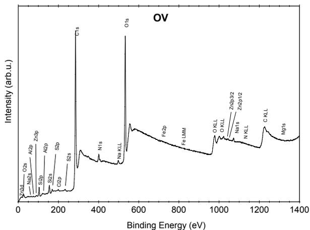
Fig. 5. Example of the XPS spectrum for the PM10 sample from “BACKGROUND” (May10-11).
