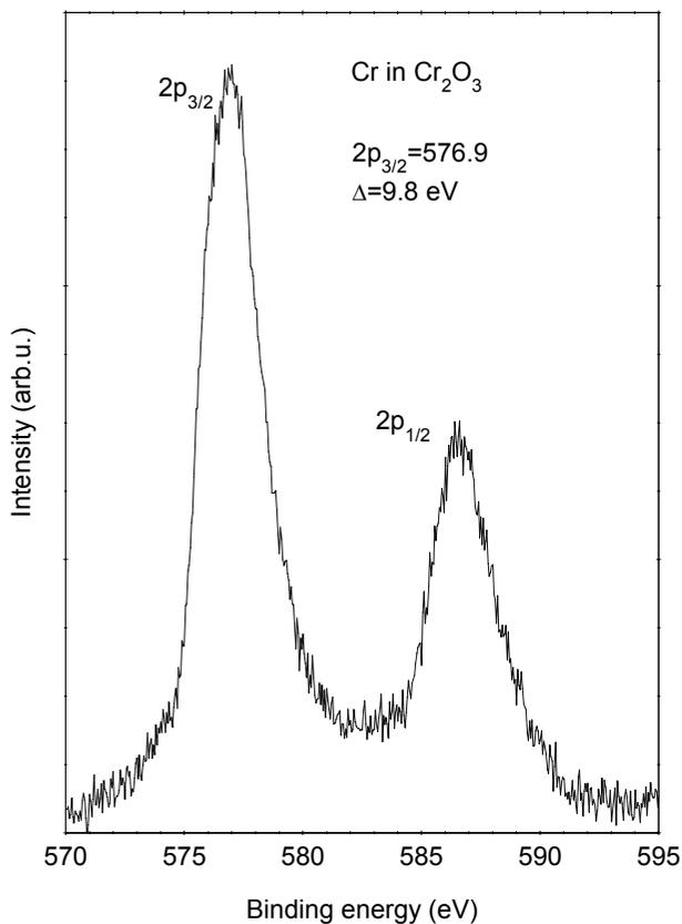
Fig. 9. Chromium spectral line in narrow energy bandwidth 570 – 595 eV for PM2.5 sampled on August 10-11, 2005, at “CROSSROADS.”
