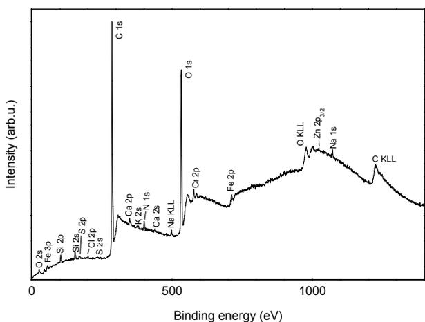
Fig. 6. Example of the XPS spectrum for the PM2.5 sample from “CROSSROADS” (August 10-11).
