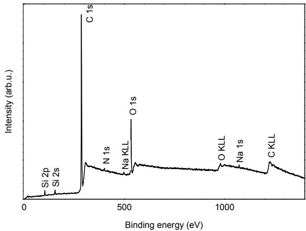
Fig. 7. Example of the XPS spectrum for the PM2.5 sample from “BACKGROUND” (August 10-11).
