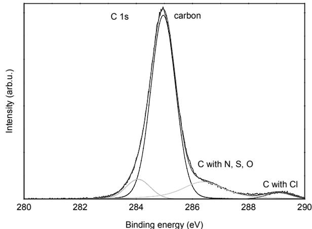
Fig. 8b. Carbon spectral line in narrow energy bandwidth 280 – 290 eV for PM2.5 sampled on August 10-11, 2005, at “CROSS-ROADS.”
