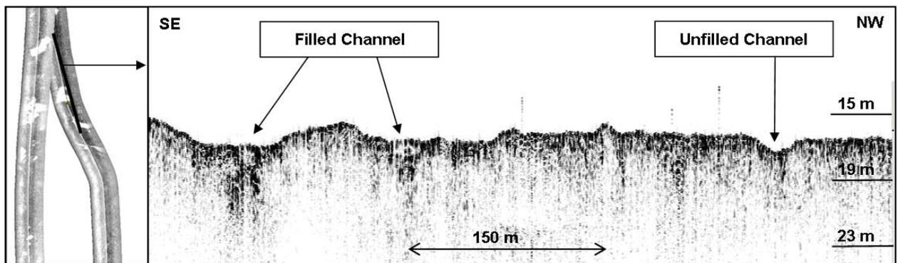
Fig. 6. Shallow seismic profiles close to the coastline with small channels. Some of these channels are filled with finer sediment, which appears white in the side scan sonar data. For the location of the figure, refer to Fig. 4.
