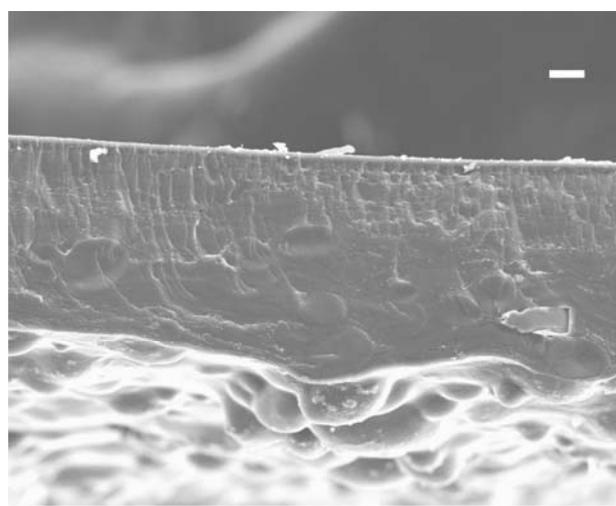
Fig. 6. Foil obtained of starch foil and glycerine as a plasticizer and montmorillonite as a filler (scale bar 20  $\mu\text{m}$ ).
