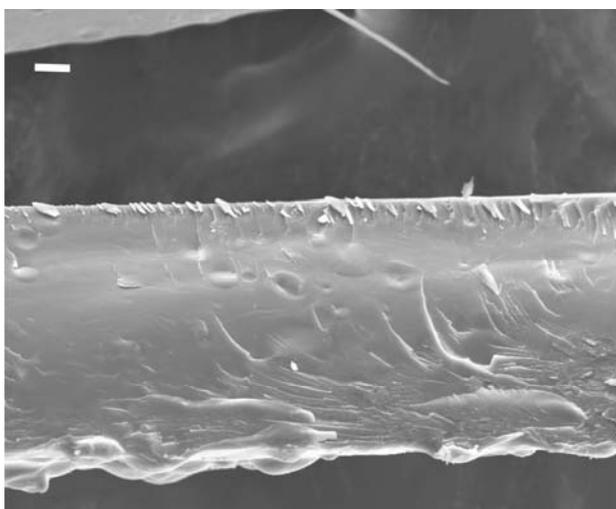
Fig. 3. Foil obtained from pure starch, with no additions (scale bar 20  $\mu\text{m}$ ).
