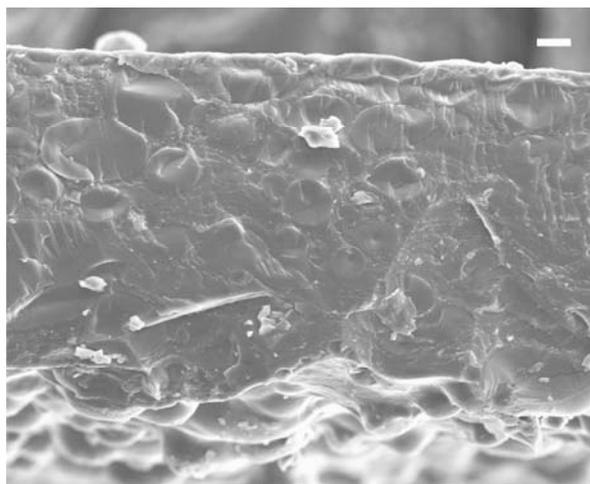
Fig. 7. Foil obtained of starch foil and glycerine as a plasticizer and bentonite as a filler (scale bar 20  $\mu\text{m}$ ).
