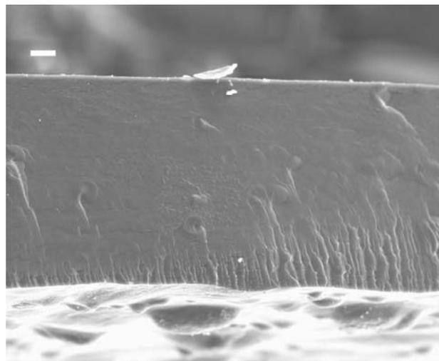
Fig. 4. Foil obtained of starch and glycerine as a plasticizer (scale bar 20  $\mu\text{m}$ ).
