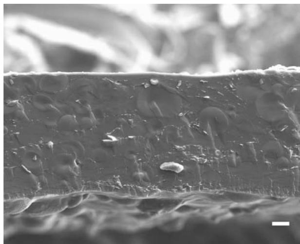
Fig. 5. Foil obtained of starch foil and glycerine as a plasticizer and kaolin as a filler (scale bar 20  $\mu\text{m}$ ).
