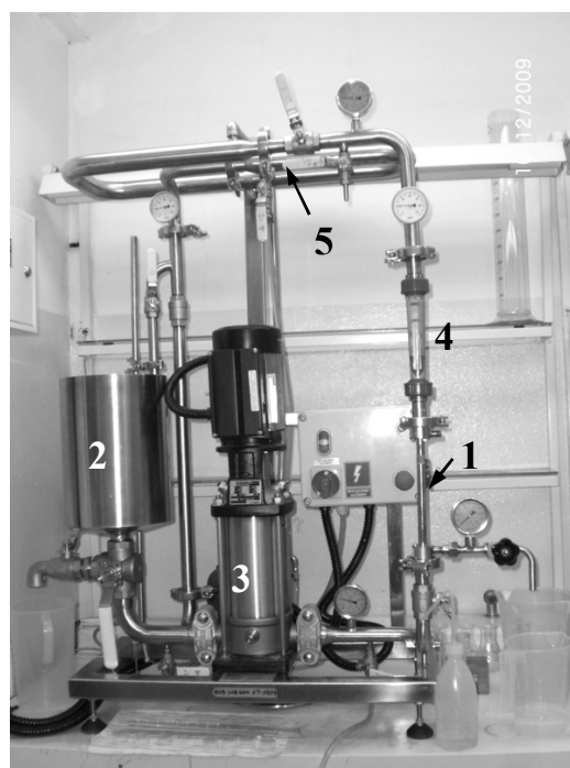
Fig. 2. Ultrafiltration cross-flow system: 1 – membrane module, 2 – feed tank, 3 – pump, 4 – flow meter, 5 – thermostat.
