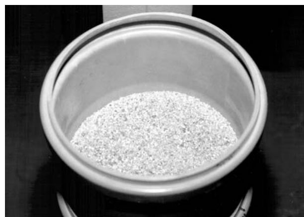
Fig. 2. The sand matrix treated by hydrocarbons in the soil filter.
