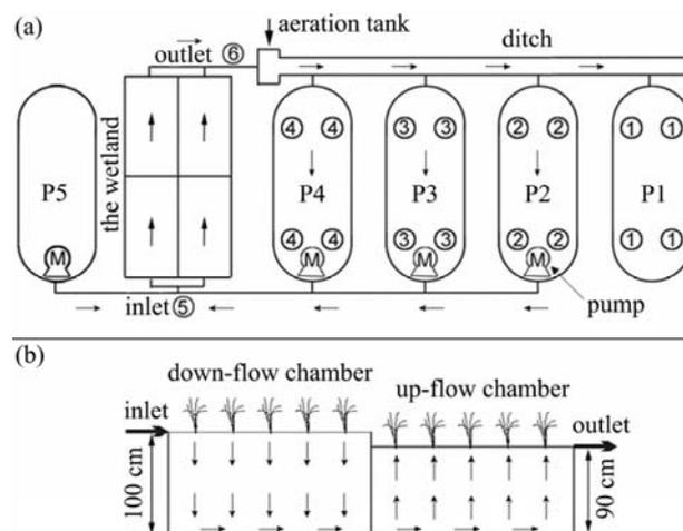
Fig. 1. Schematic diagram of the RAS (a) and the CWs (b); P1-P5 represent five culture ponds and numbers of 1-6 in circles represent sampling sites; arrows show water flow direction.
