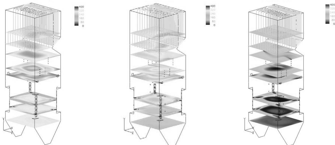
Fig. 9. NO x contours of (left) baseline with LNB, (middle) coal-only ROFA and (right) biomass ROFA.
