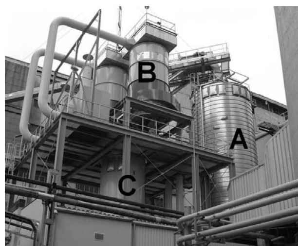
Fig. 2. Overview of Biomass Handling System: (A) Pellet Silo, (B) Cyclone Filters, and (C) Powder Silo.
