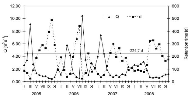
Fig. 4. Relationship between the amount of water flowing into the Słup Reservoir and reservoir capacity in a given time vs. changeability of the retention time, 2005-08.
