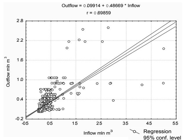
Fig. 5. Graphical presentation of the correlation between the volume of outflowing and inflowing water in the Słup Reservoir ( $Q_{\text{out\_res}}$  and  $Q_{\text{in\_res}}$ ), 2005-08.
