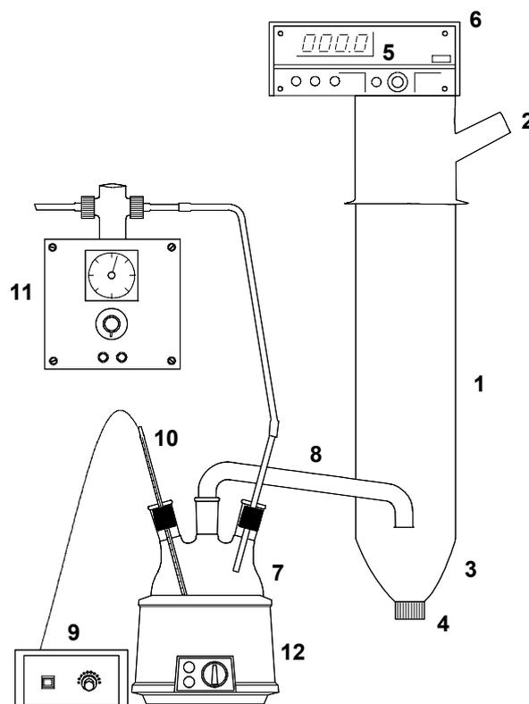
Fig. 2. The hydrophobization apparatus scheme: 1 – hydrophobization column, 2, 3 – hoppers, 4 – lock of hopper, 5 – control panel, 6 – feeder, 7 – boiler, 8 – ting-up pipe, 9 – thermoregulator, 10 – thermocouple, 11 – compressor, 12 – heater.
