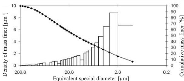
Fig. 1. Curve of grain distribution for raw dust.
