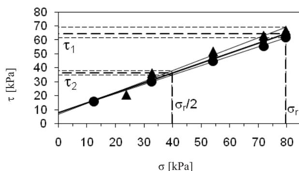
Fig. 3. Relations of shear stress-normal stress of tested materials (■ – raw, ● – S\_18, ▲ – S\_SH15).
