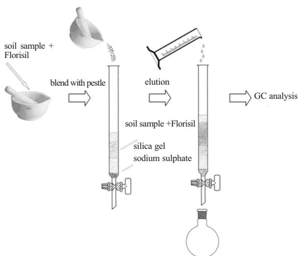
Fig. 2. Steps in soil sample extraction by MSPD and clean-up by column chromatography.
