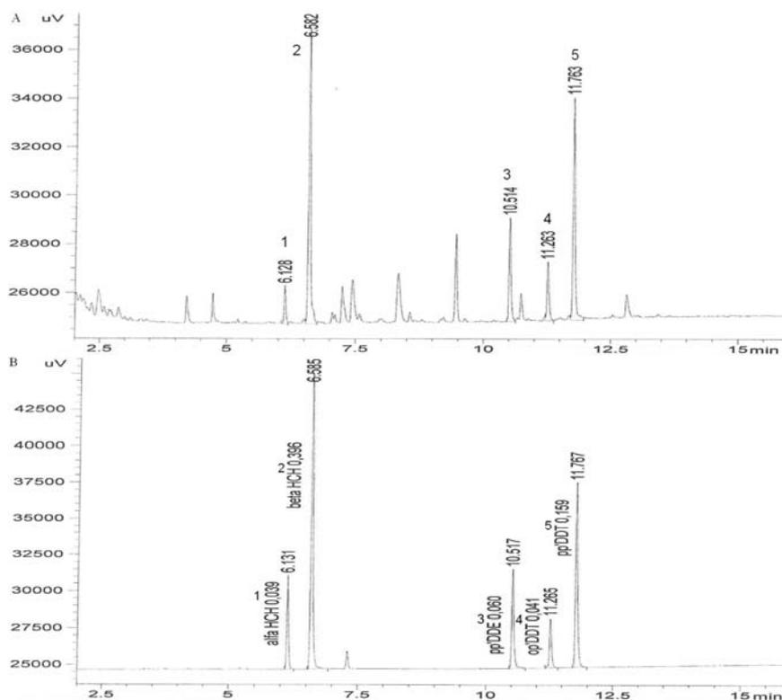
Fig. 6. GC chromatogram of A: CRM soil sample – 1. alfa-HCH; 2. beta-HCH; 3. p,p'DDE; 4. o,p'DDT; 5. p,p'DDT and B: standard mixture – 1. alfa-HCH (0.005 mg/kg); 2. beta-HCH (0.01 mg/kg); 3. p,p'DDE (0.005 mg/kg); 4. o,p'DDT (0.005 mg/kg); 5. p,p'DDT (0.005 mg/kg) (HP-5 column).
