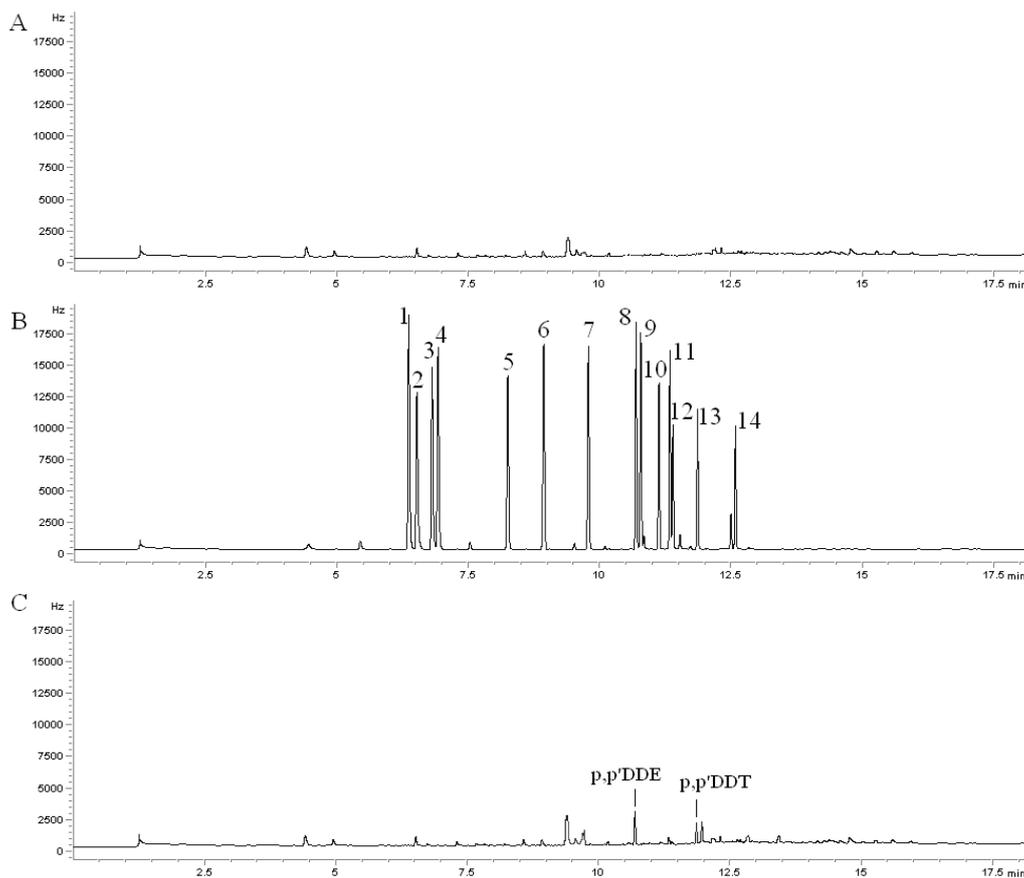
Fig. 7. Chromatograms of: A: blank soil sample, B: selected standards mixture – 1. alpha-HCH; 2. HCB; 3. beta-HCH; 4. gamma-HCH; 5. heptachlor; 6. aldrin; 7. heptachlor-epoxide; 8. p,p'DDE; 9. dieldrin; 10. endrin; 11. p,p'DDD; 12. o,p'DDT; 13. p,p'DDT; 14. metoxychlor (DMDT) and C: field soil sample with detected p,p'DDE  $0.007 \pm 0.0006$  mg/kg ( $t_R = 10.519$  min) and p,p'DDT  $0.009 \pm 0.0006$  mg/kg ( $t_R = 11.768$  min) (HP-5 column).
