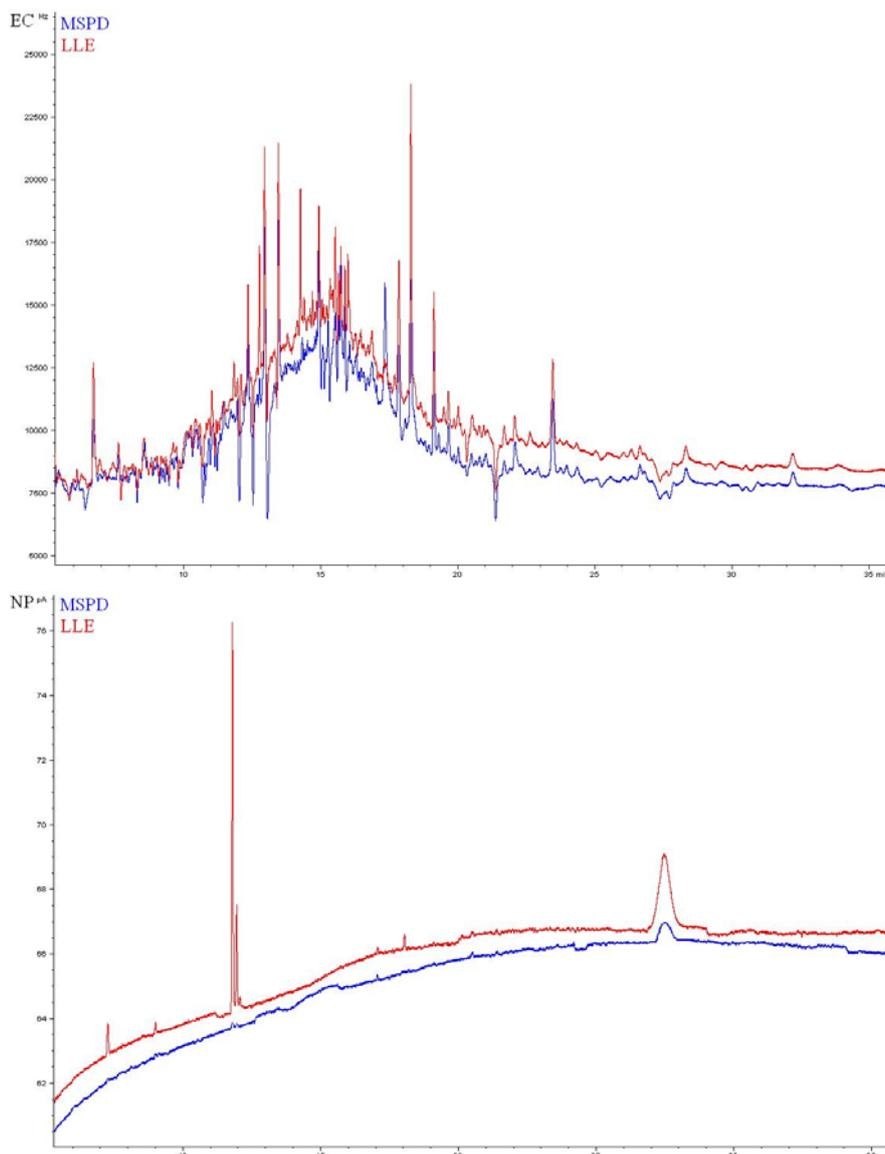
Fig. 5. EC and NP chromatograms of blank soil sample from both extraction procedures MSPD and LLE (DB-35 column).
