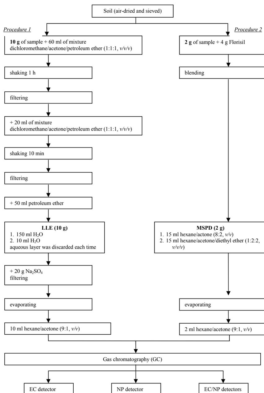
Fig. 1. Scheme of the LLE and MSPD extraction procedures for isolation and purification of pesticides from soil samples.
