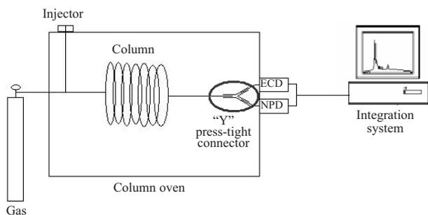
Fig. 3. GC with dual system EC/NP detectors scheme.
