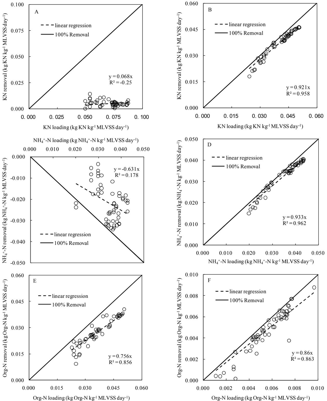
Fig. 4. KN NH<sub>4</sub><sup>+</sup>-N Org-N loading and removal rates of two subsystems.
