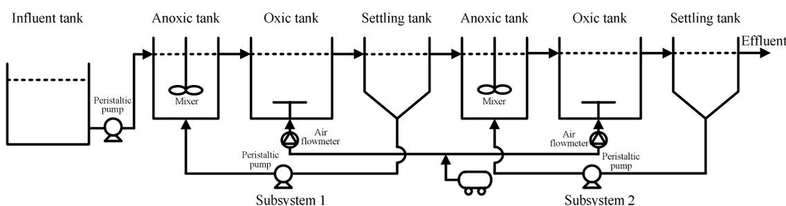
Fig. 1. A schematic diagram of two-stage A/O system.
