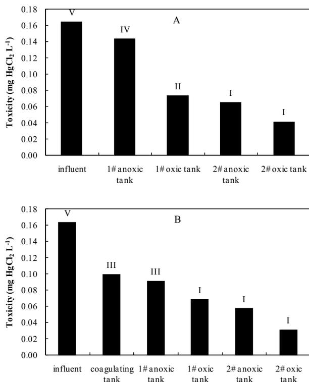
Fig. 5. Wastewater acute toxicity of different units in a two-stage A/O system.
