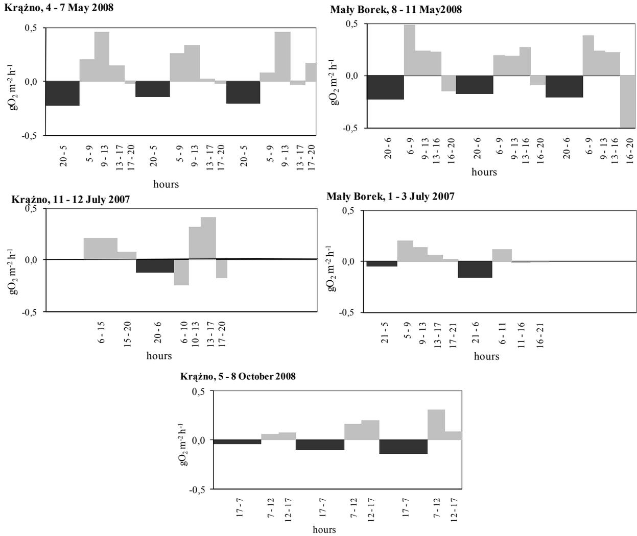
Fig. 6. Rates of oxygen concentration changes (gO<sub>2</sub>·m<sup>-2</sup>·h<sup>-1</sup>) in lakes Krażno (left) and Mały Borek (right); dark columns are night.
