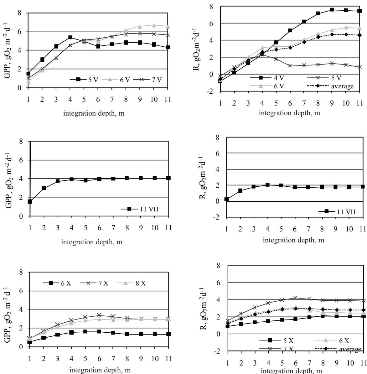
Fig. 8. Dependence of GPP and R values on the depth of data integration in lake Krężno; (May and October – data from 2008, July – data from 2007).
