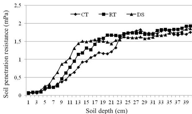
Fig. 3. Soil penetration resistance as a function of tillage depth and tillage methods.
