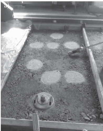
Fig. 2. a) Static Plate Load Test in situ
